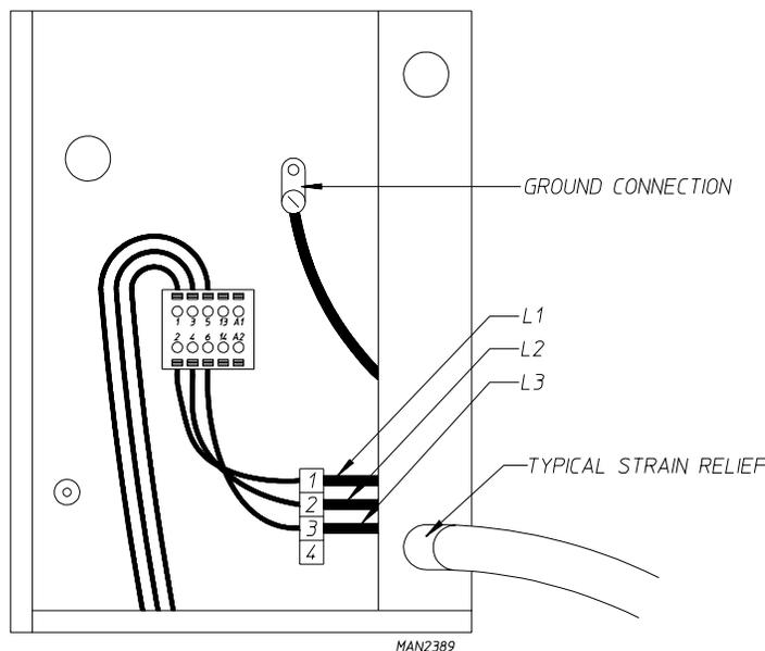
**CAUTION:** The dryer **must be** grounded. A ground lug has been provided for this purpose.
