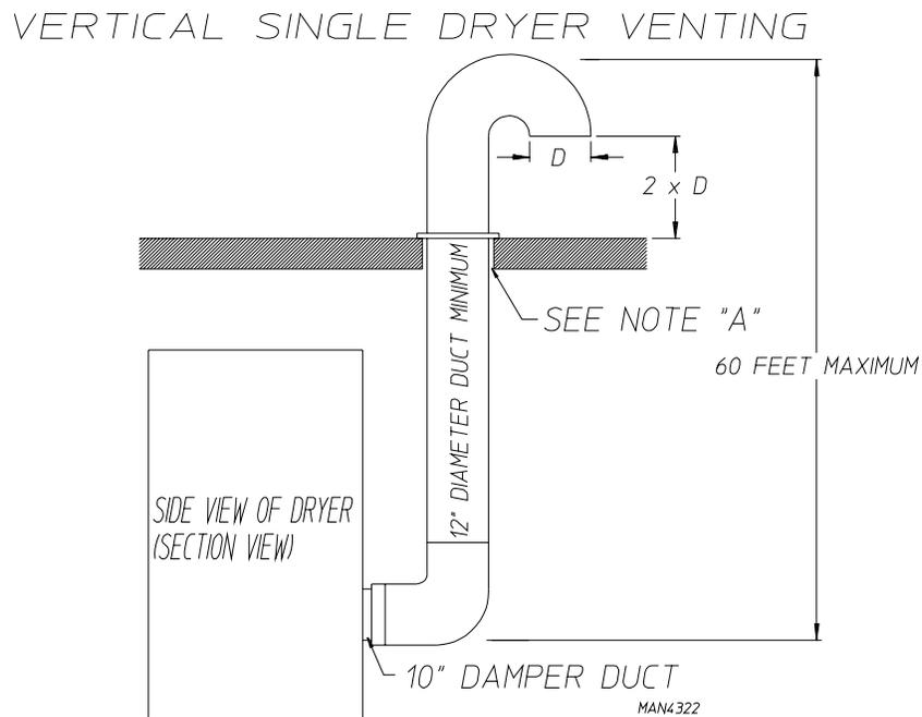
NOTE A: OPENING MUST BE TWO (2) INCHES LARGER THAN THE DUCT (ALL THE WAY AROUND)
