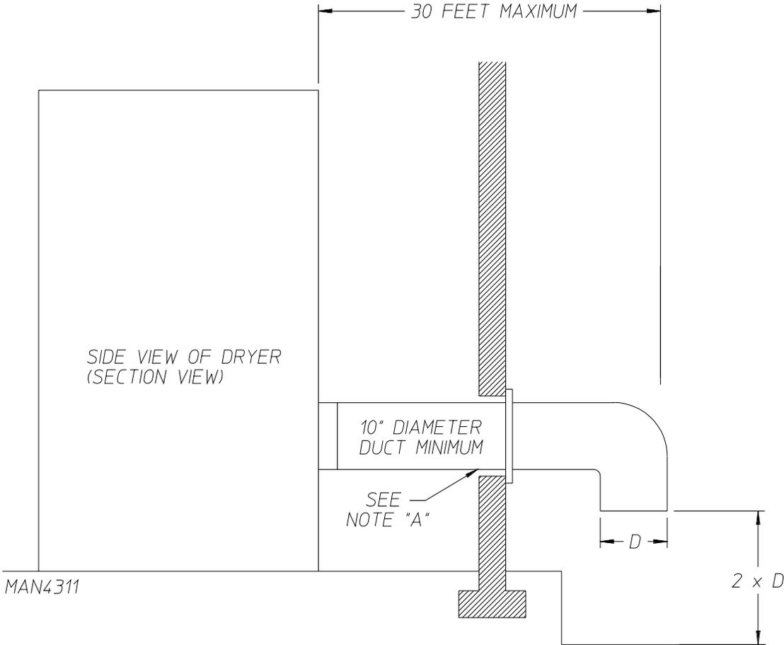
NOTE A: OPENING MUST BE TWO (2) INCHES LARGER THAN THE DUCT (ALL THE WAY AROUND) THE DUCT MUST BE CENTERED WITHIN THIS OPENING.
