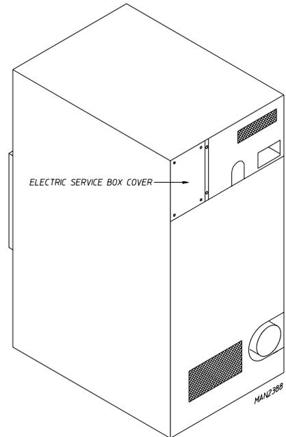
Providing local codes permit, power to a gas dryer can be made by the use of a flexible U.L. listed power cord or pigtail (wire size **must conform** to rating of dryer), or the dryer can be hard wired directly to the service breaker panel. In **ALL** cases, a strain relief **must be** installed where the wiring enters the dryer and service box area.
