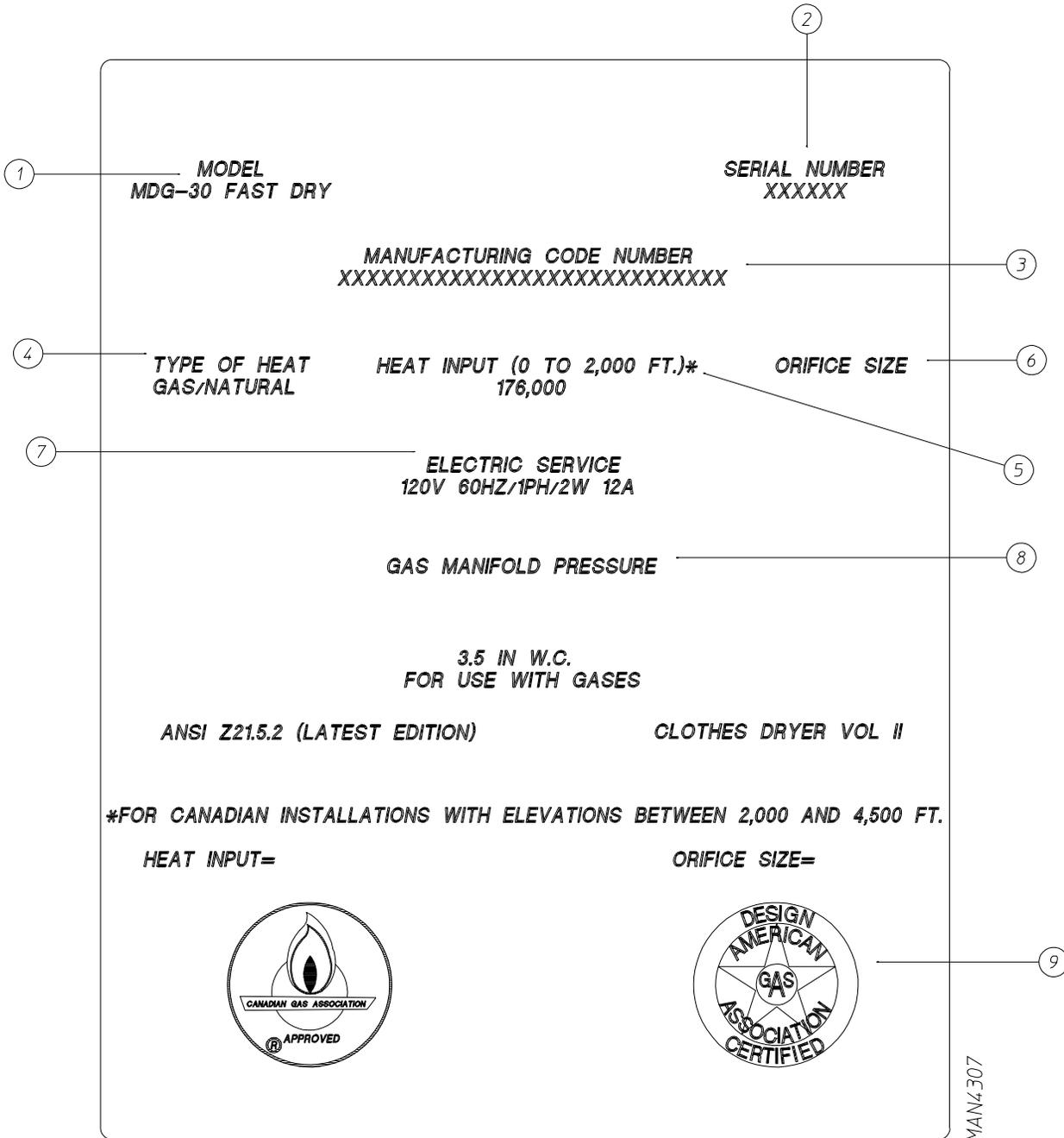
When contacting the **Maytag Co.** certain information is required to ensure proper service and parts information from the manufacturer. This information is on the data label located on the inside of the control door. When contacting the **Maytag Co.** please have the **model** and **serial numbers** available.
